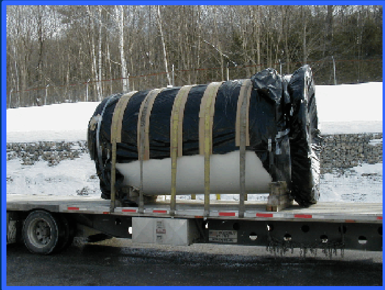
Dry storage liner in transit to reactor site
