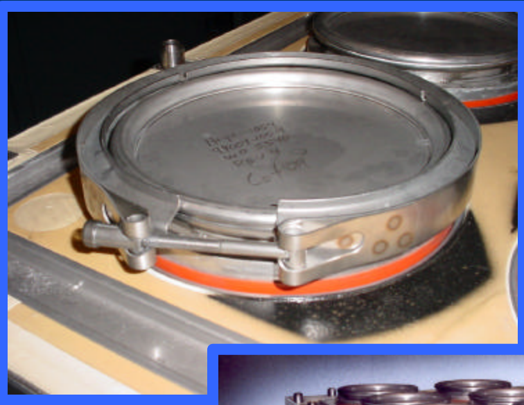
ICCA with Locking Ring Inserted into New Powder Container (NPC)
