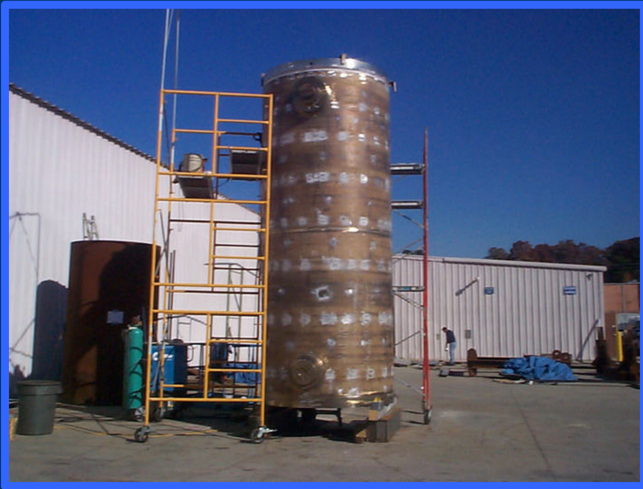
Transfer cask in manufacturing with interlocking lead brick shielding
