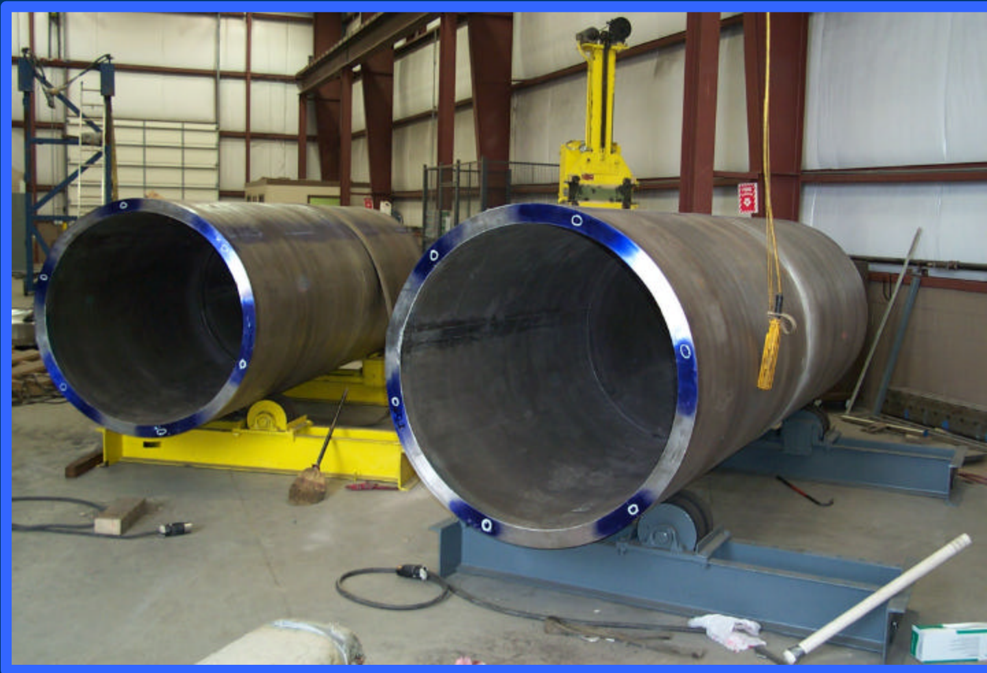
Greater Than Class C canister shells in process
