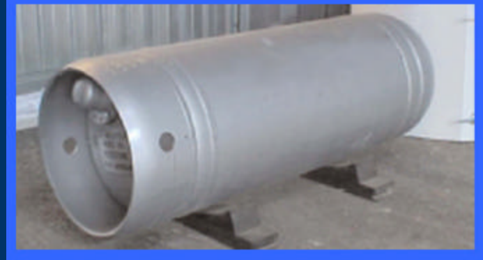
Watertight technology on enriched UF 6 cylinder
