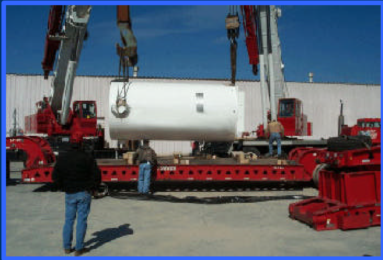
Transfer cask being loaded
