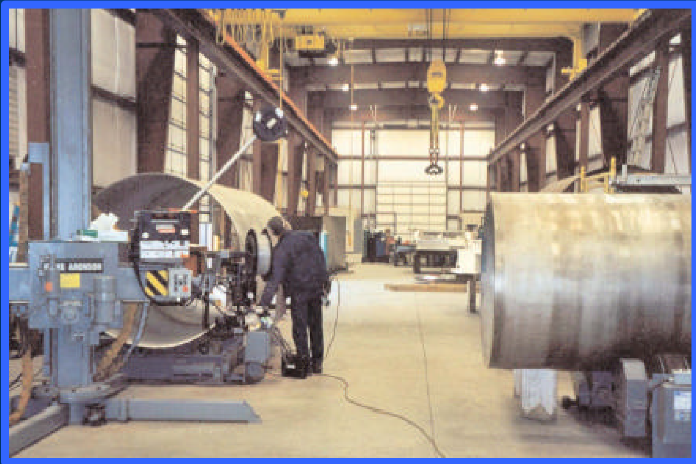
Stainless Canister Shells in manufacturing
