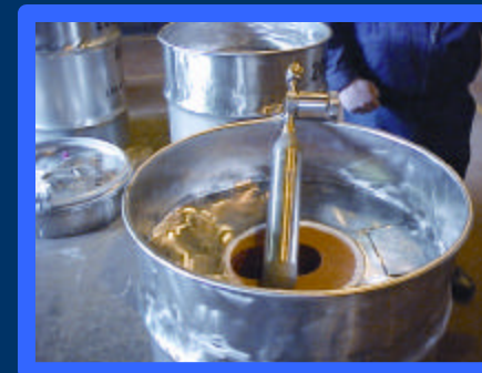
MED 2000 is for enriched UF 6 sample bottle packages
