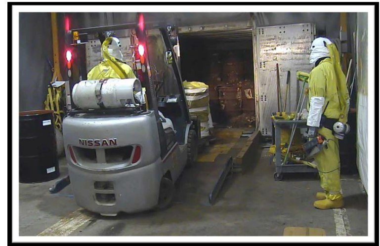
Retrieval of legacy drums from AMWTP cargo container for processing (~30 of 104 cargo containers emptied)
