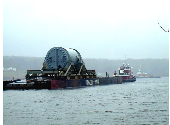
Reactor Pressure Vessel Shipping at Maine Yankee
