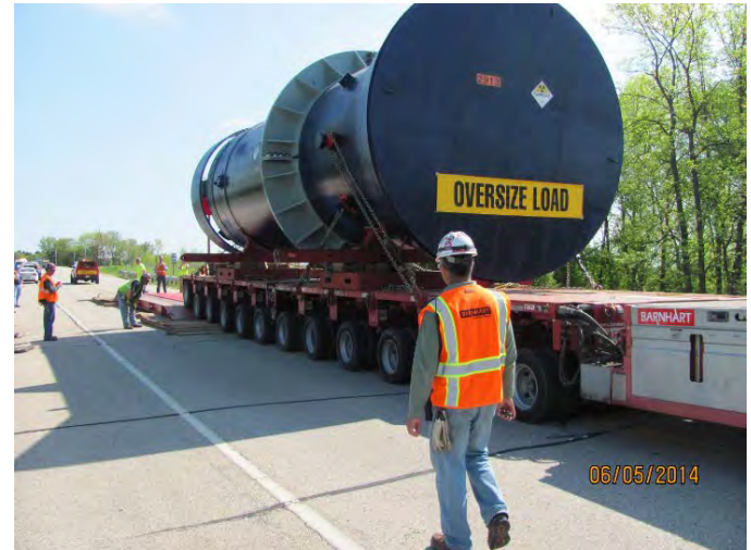
Steam Generator Shipping Near Kewaunee
