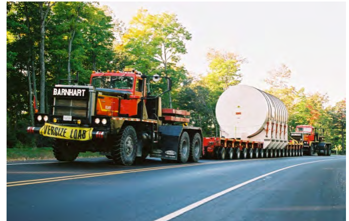
Big Rock Point Reactor Pressure Vessel Heavy Haul
