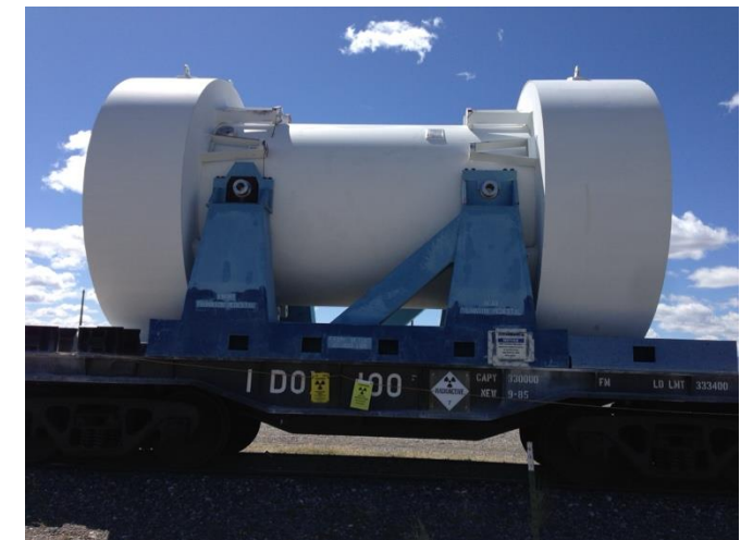
A cutaway figure of a transportation cask (top) and a transportation cask with impact limiters loaded on a railcar (bottom).
